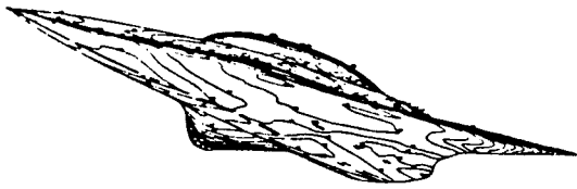
Bild 1a: Non-radiating adiabatic wall. T_{\min} = 1. , T_{\max} = 10.3 , \Delta = 0.2 .
