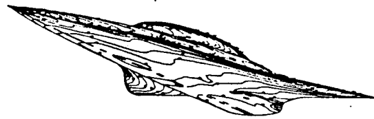
Bild 1b: Radiating adiabatic wall, \epsilon = 0.85 . T_{\min} = 1. , T_{\max} = 7.7 , \Delta = 0.2 .
