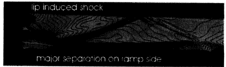
Fig.1 Superposition of an experimentally obtained Schlieren picture [2] showing the density gradients and the computed contour plot of Mach number distribution for a M_0=3.0 with major separation on the ramp side.
