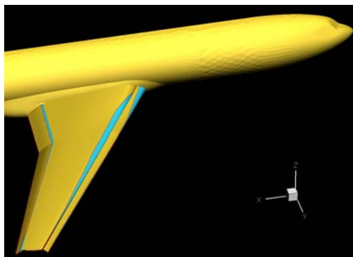
Fig. 4 Laminar regions on the upper sides of all three wing elements of a wing-body high-lift configuration.
