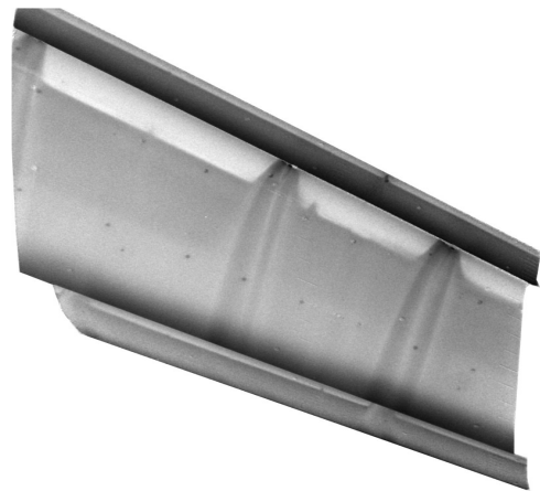
Figure 2: Transition patterns on a half model wing tested in the ETW wind tunnel by means of cryoTSP. Dark areas represent turbulent and bright areas laminar boundary layer state.
