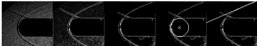
Figure 1: Example of position detection of a Pitot pressure probe and the far field shock shape angle in HEG.
