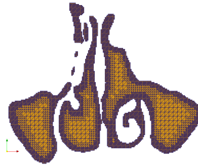
Fig. 3: Slice through the computational grid of the nasal cavity with local grid refinement.
