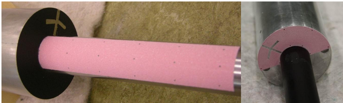
Fig. 1 Close-up on the model of the generic space launcher made from aluminum and covered with unsteady pressure-sensitive paint (iPSP). The model is equipped with unsteady pressure and temperature sensors; left: coating for sting investigations; right: coating for base investigations
