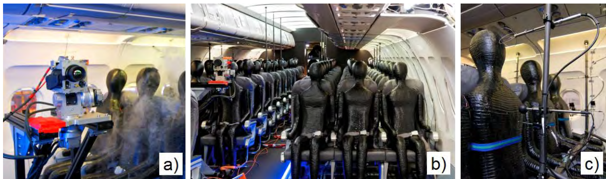
Fig. 1: Cabin flight test installation for investigation of CDV. a) Automatically turnable IR camera with thermal passenger dummies, b) thermal passenger dummies, measurement racks, IR camera during installation and c) thermal passenger dummies with measurement racks.
