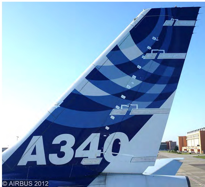
Fig. 1: Installation of Vortex Generators at the VTP of A340-600
