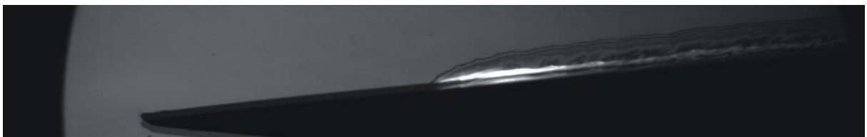
Figure 2: Electric discharge generated on a flat plate; U_\infty=40 m/s, \alpha_0=-5^\circ , stored electric energy 96 J, current limitation 10 A.
