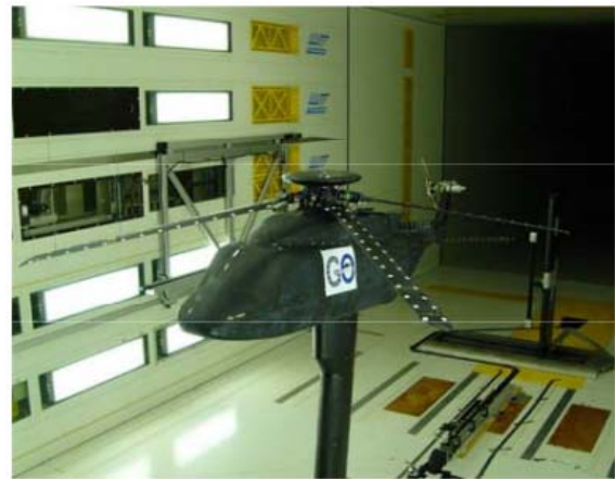
Figure 1: GOAHEAD wind tunnel model [1]
