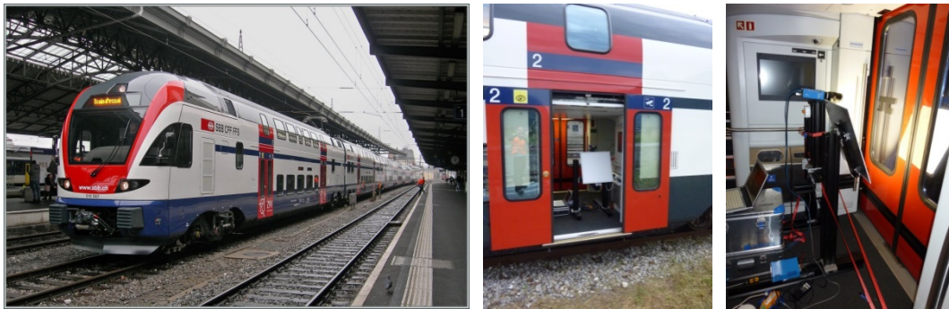
Figure 1. Electric double-deck train KISS (left), measuring position in the first car (middle) and experimental setup consisting of a CCD camera and a LED panel (right).
