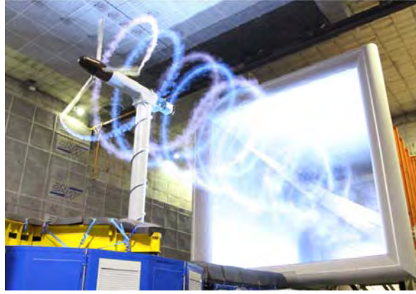
Figure 1: New MEXICO rotor experiment in the DNW-LLF – smoke visualization of the blade tip vortices under axial flow conditions (Photo from Boorsma, K.; Schepers, J.G.; “Description of Experimental Setup”, ECN, 2015).
