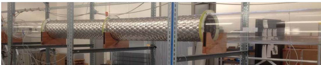
Fig.(4) two meters long structured segment mounted in the Colapipe at L/D = 113.
