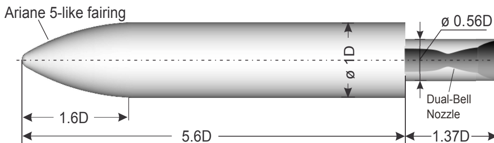
Figure 1: Geometry parameters of the investigated generic planar transonic configuration
