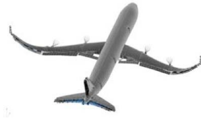
Aero-elastic deformation (amplified) of an aircraft in cruise
