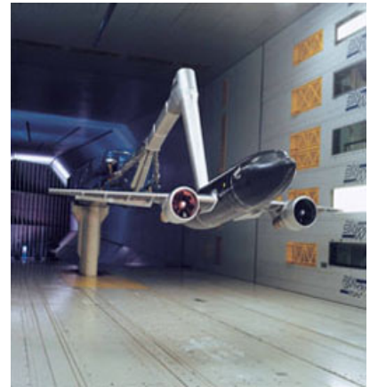
Wind tunnel test at DNW (LLF, Nordoostpolder, Niederlande)
