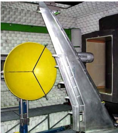
Aero-acoustic measurement on a half wing model
