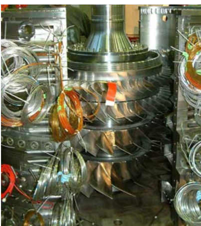
Four-stage transonic compressor of the DLR
