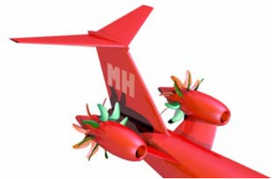
Integration of new propulsion concepts at the rear fuselage
