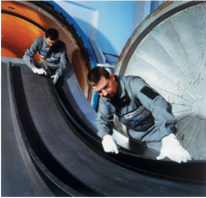
CFRP shell element in front of an autoclave at the DLR
