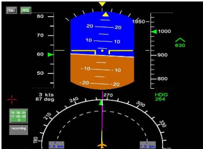
Extended primary flight display with additional guidance cues for flying predefined 4D missions
