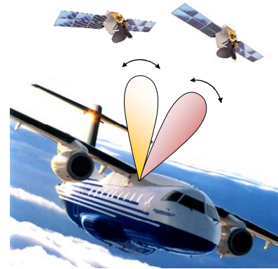
Electronically steerable antenna array for satellite navigation or communication.
