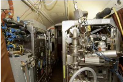
Instrumentation for air pollution measurements inside a research aircraft
