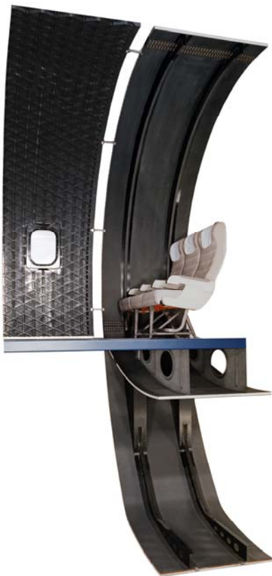
Concept of a CFRP fuselage segment structure
