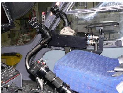
FHS-cockpit with integrated active sidestick
