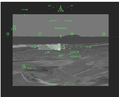
Enhanced vision display for approaches under poor visual conditions
