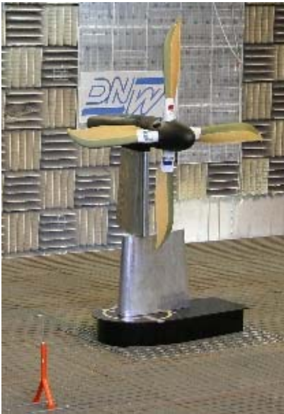
TILTAERO tilt rotor model in DNW LLF
