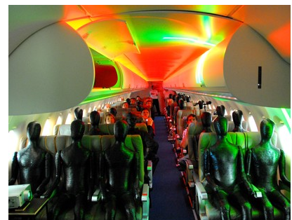
On-board climate measurement installation in an aircraft cabin
