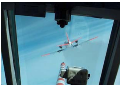
Measuring the exhaust of ATTAS from the DLR's Falcon
