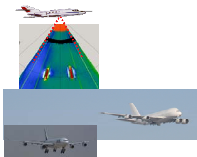
Simultaneous measurement of the wake vortices of an A380 and A340 with a Lidar on board the Falcon research aircraft
