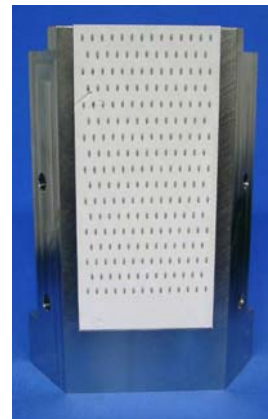
WHIPOX segment with cooling channels for a model combustion chamber
