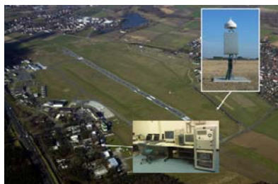
GBAS-station in Braunschweig.
