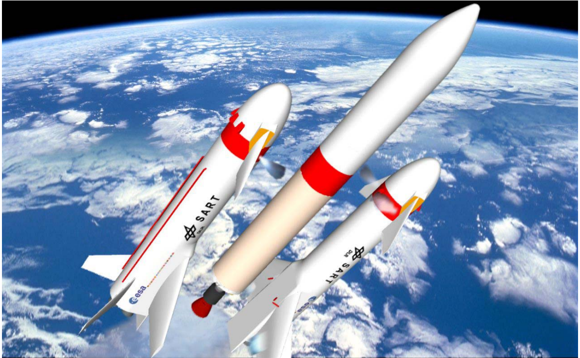
Figure 1: Artists impression of the separation of two attached reusable fly-back boosters from the Ariane 5 core stage
