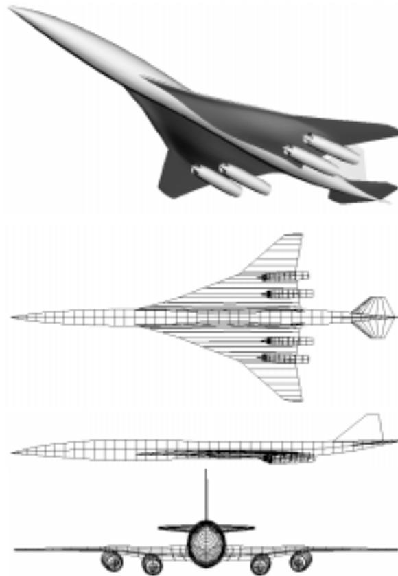
Fig. 8: "Configuration 950" Generic HSCT configuration derived from Boeing Mach 2.4 test case
