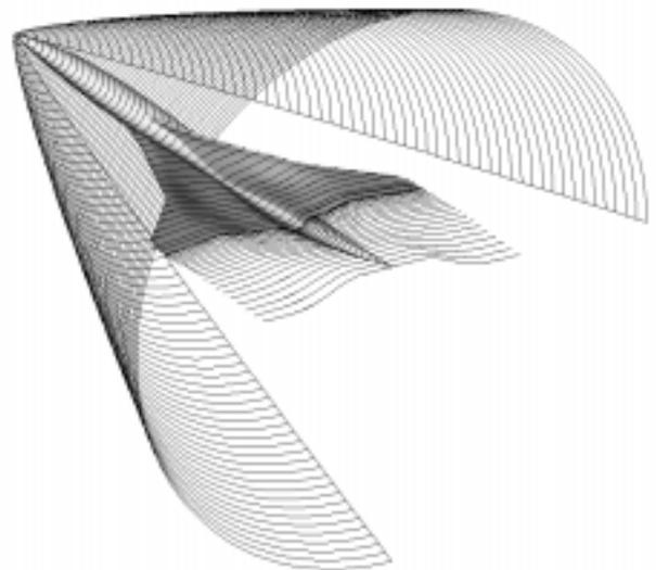
Fig. 10: Cross sections of wing-body, far field boundary and a computational wake model.
