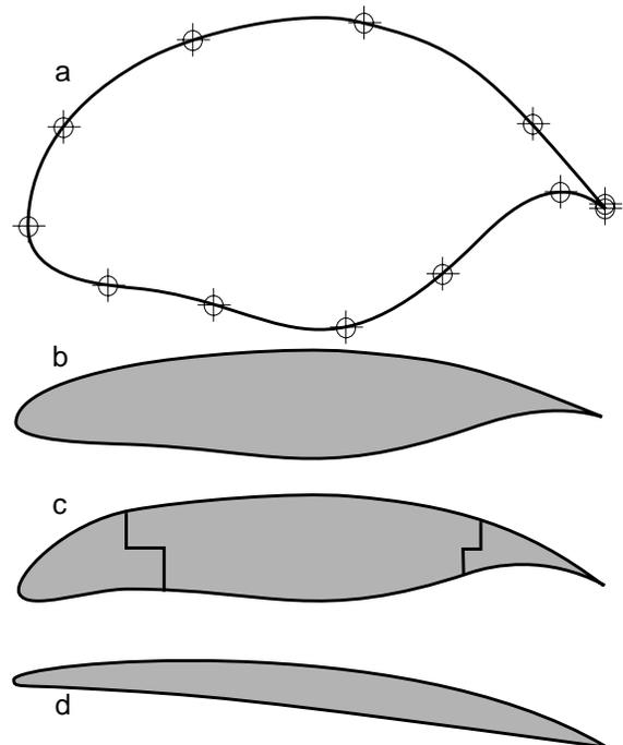
Fig. 3: Airfoils given as datasets either with few supports in blow-up scale (a) or from external database; with additional parameters for local deformation (b  $\rightarrow$  c) and as analytical functions, for standard airfoils or guided by known flow field solutions (d).
