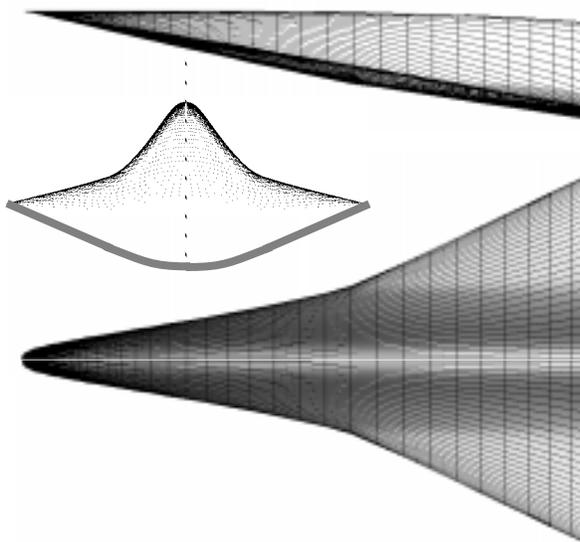
Fig. 7: Waverider wing configuration designed from given leading edge, Mach number and oblique shock wave angle. Supersonic leading edge and a completely integrated body are trademarks of waverider configurations.
