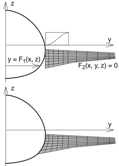
Fig. 5: Combination of two components by a blended projection technique
