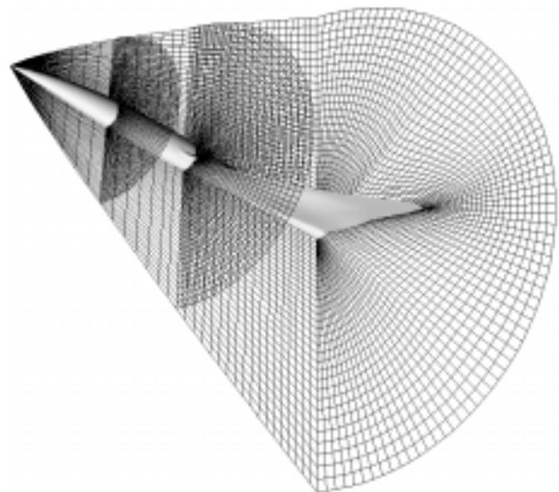
Fig. 11: Algebraic grid (33 x 81 x 33) for preliminary CFD analysis near design conditions.
