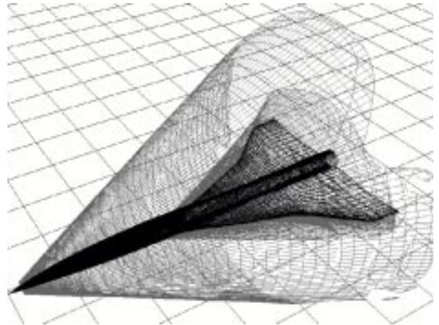
Fig. 14: Visualization of the shock system emanating from body tip and wing.
