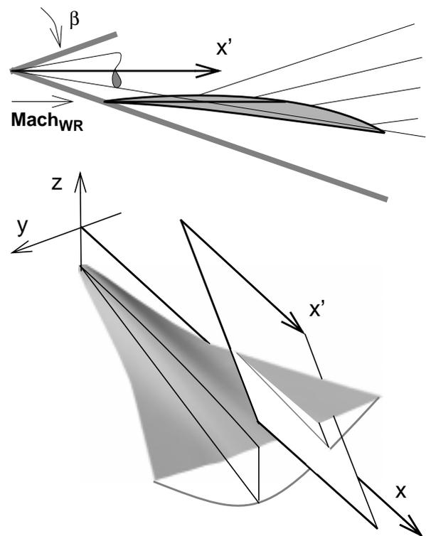
Fig. 6: Exploiting known supersonic flow fields to design wing sections (above) and using osculating cones concept to design waverider wings (below).
