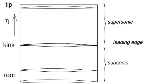
Fig. 9: Airfoil support shapes along span.
