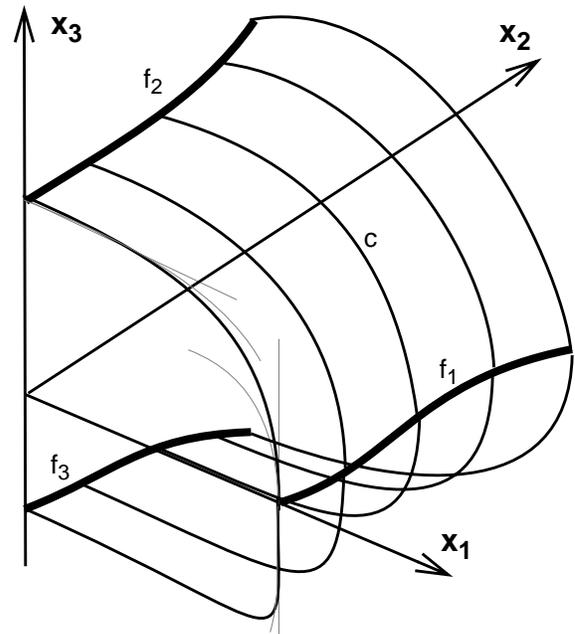
Fig. 2: Surface definition by cross sections  $c$  in plane  $(x_1, x_3)$  determined by generatrices  $f_i$  along  $x_2$  and in planes  $(x_1, x_2)$ ,  $(x_2, x_3)$ .
