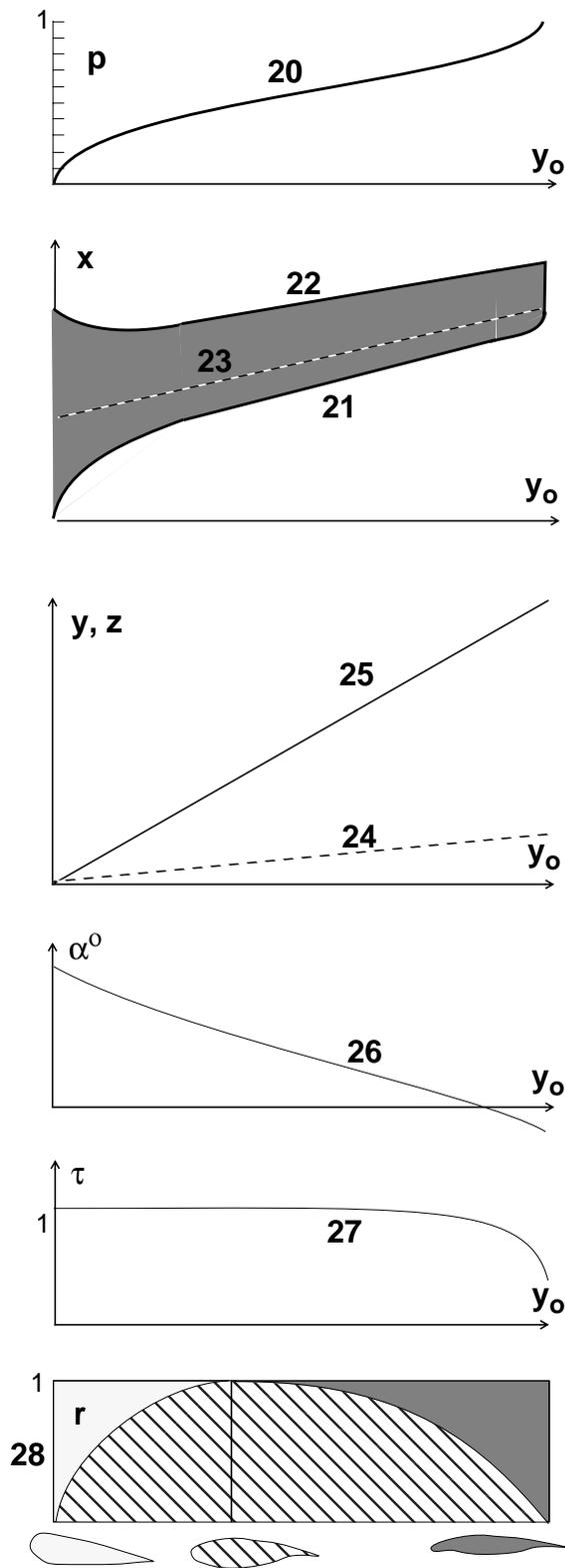
Fig. 4: Wing parameters and respective key numbers for section distribution, planform, an/dihedral, twist, thickness distribution and airfoil blending.
