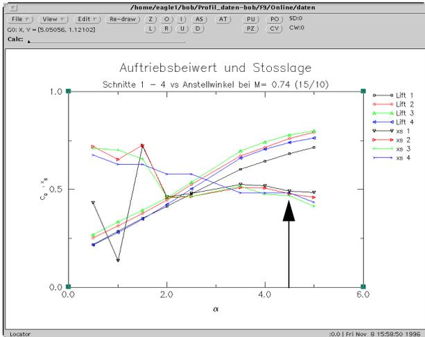
Figure 12: Lift coefficient and shock location vs. angle of attack, four wing sections. (Flow parameters equivalent to Figure 11)
