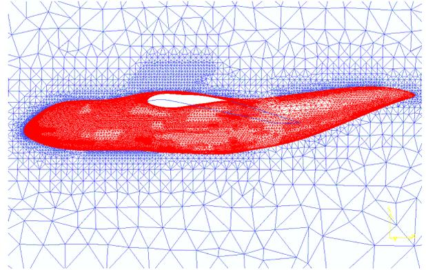
Figure 8: Unstructured grid for Euler flow simulation.
