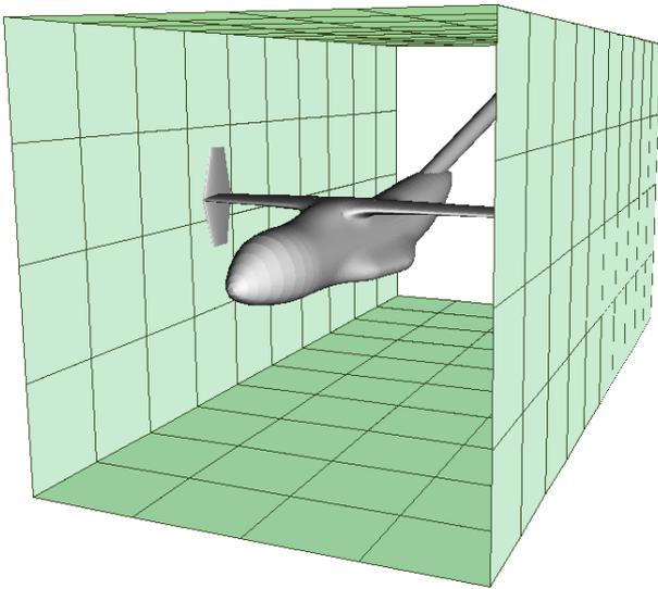
Figure 7: DLR-F9: general arrangement in TWG wind tunnel.
