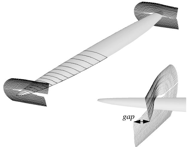
Figure 4: Stream surfaces past elliptic wing at 90% of halfspan, larger gap resulting from higher lift.
