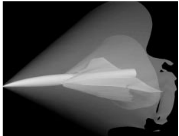
Figure 3. Shock system emanating from a wing - body configuration in supersonic flow Mach = 2.4. Visualization of CFD Euler result with cut off shock surface at defined shock strength threshold
