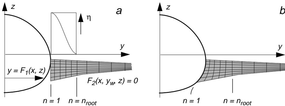
Fig. 2. Blended projection technique to mount a wing  $F_2$  onto a body  $F_1$ . Shape  $F_1$  remains unchanged while a portion of  $F_2$  is moved into  $y$ -direction controlled by blending function  $\eta(n)$ .
