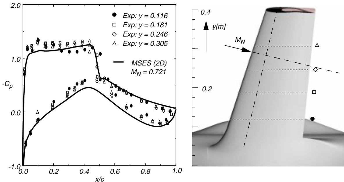
Fig. 9. Experimental results for DLR-F9 configuration in transonic wind tunnel at  $M_\infty = 0.74$ : Pressure measurements in 4 wing sections at optimally adjusted circulation control: pressure distribution and shock position close to isobar design concept of the wing.
