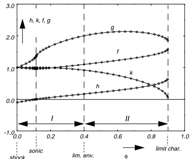
Fig. 5. Functions  $h, k, f, g$  for a conical flow example. The solution contains two flow models: (I) transonic accelerated and (II) supersonic decelerated conical flow
