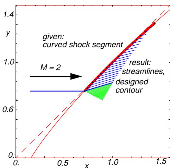
Fig. 9. Computation of an axisymmetric flow with curved shock wave. Shock angle varies from  $50^\circ$  to  $40^\circ$
