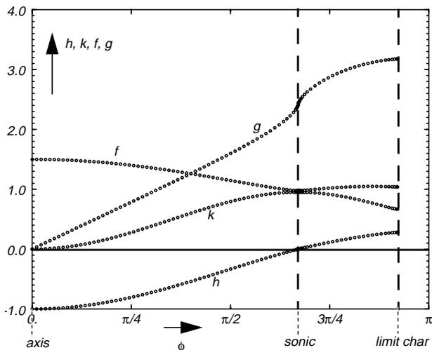
Fig. 3. Functions  $h, k, f, g$  for the sonic throat example within the domain of subsonic flow and supersonic flow upstream of the first limiting characteristic.
