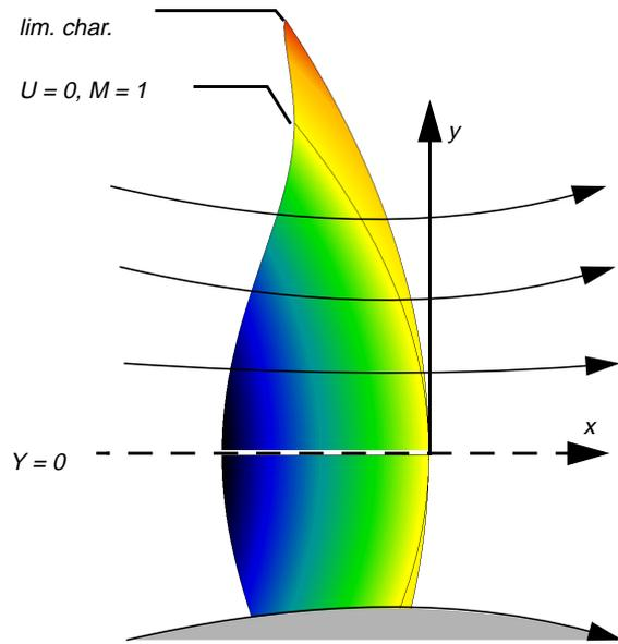
Fig. 4. Visualization of the solution for the sonic throat model. The flow is regular at the limiting characteristic and continues smoothly further downstream.
