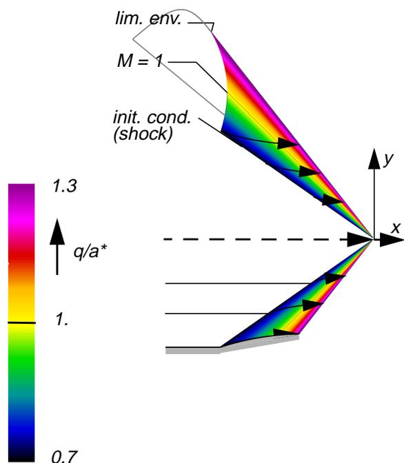
Fig. 6. Conical accelerated flow: Flow domain bounded by subsonic inlet conditions (for instance past conical shock) and singular exit condition with infinite gradients.
