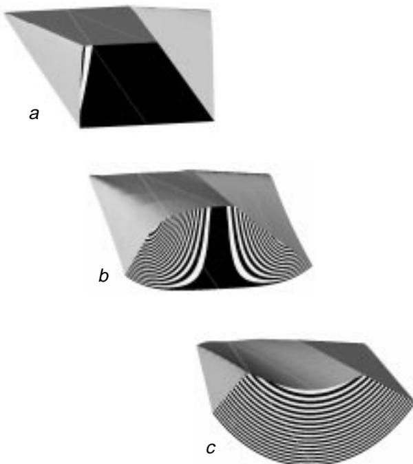
Fig. 10. Examples of inlet design using the Osculating Cones (OC) concept: Plane 2D wedge flow (a), conical flow (c) and an OC blending between a and c resulting in a geometry (b) with strong inlet flow quality control (see isobar fringes)
