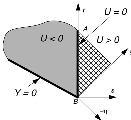
Fig. 2. Combined solution for the elliptic (subsonic) and hyperbolic (supersonic) equations, with common data (X\*, Y\*, V\*) along the sonic locus U\* = 0: Initial values define solution within triangular domain of dependence H. Characteristic variables ξ, η.
