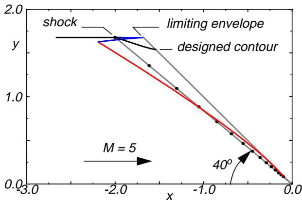
Fig. 8. Internal conical flow model with oblique shock approaching the axis, computation of the flow past given shock, resulting in contour streamline, limiting envelope and fold-back solution.
