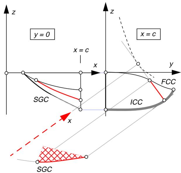
Fig. 11. Design concept of Osculating Axisymmetry. Given shock generatrix curve SGC, inlet capture curve ICC and flow capture curve FCC defines shock wave. Application of inverse method of characteristics in selected osculating planes. Varying axial distance defined by ICC curvature.
