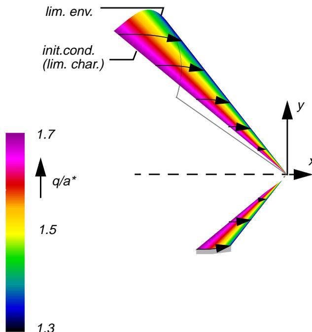
Fig. 7. Conical decelerated flow: Flow domain bounded by nearly parallel supersonic flow inlet conditions and singular exit condition with infinite gradients.
