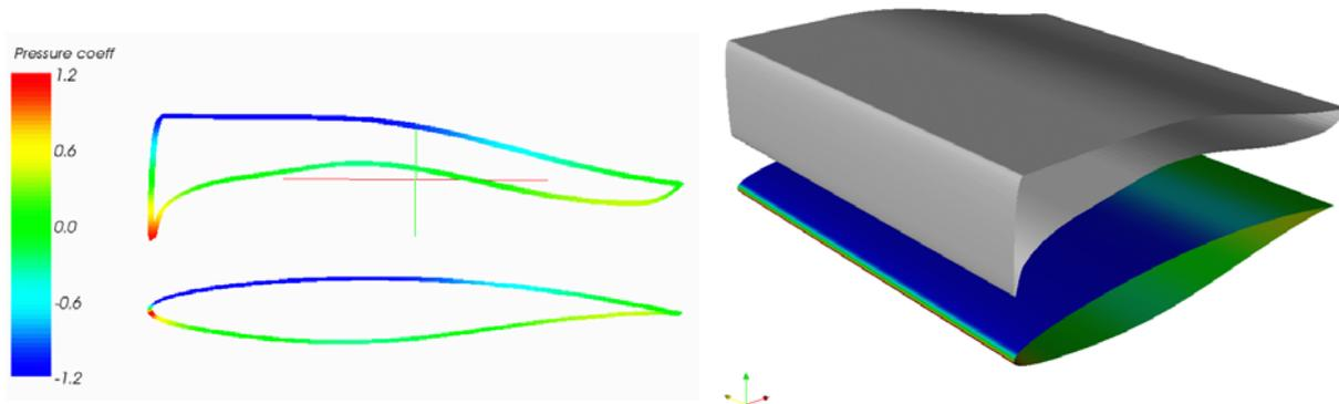
**Figure 2. PARSEC airfoil and PARCPX pressure distribution**
