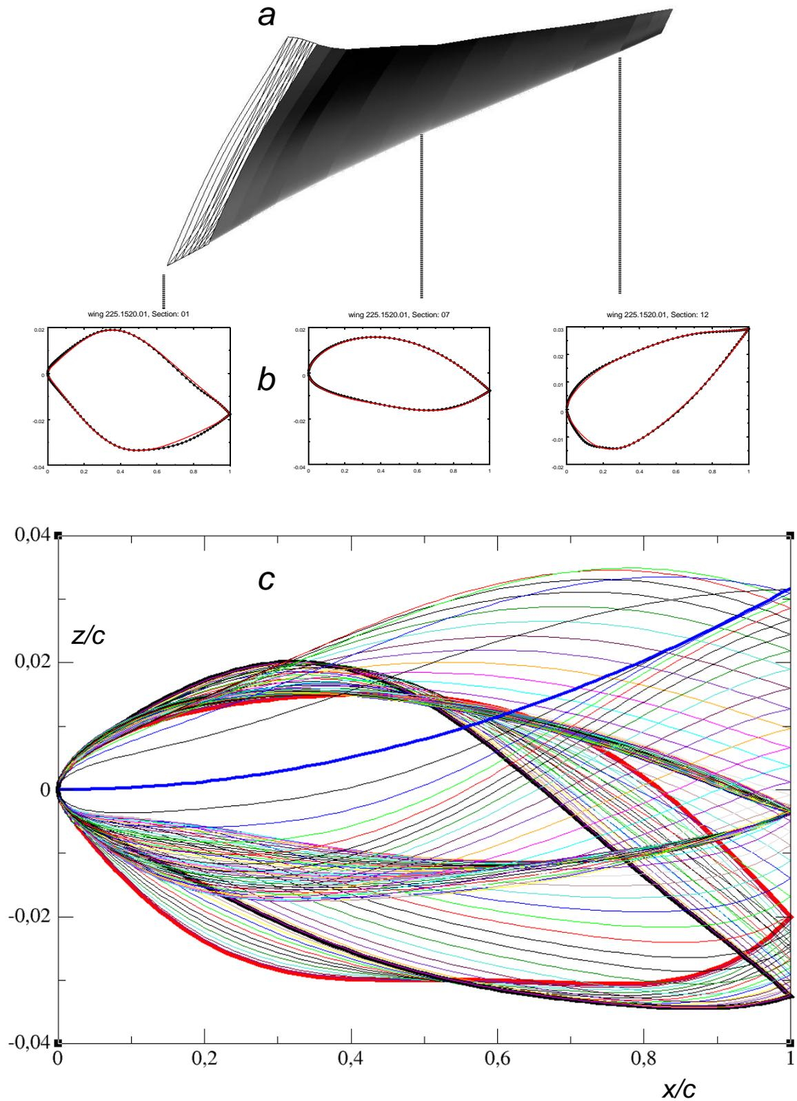
**Figure 3. Geometric redefinition of the NEXST SST wing surface**
