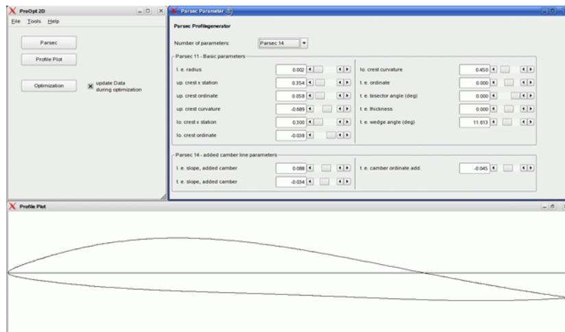
**Figure 1. PARSEC interactive code for numerical airfoil optimization [8]**
